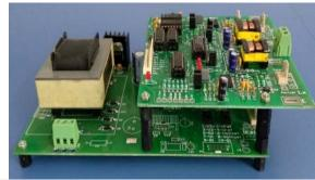
Two IGBT driver and power card for half-bridge inverter or DC-DC converter applications. It is suitable for 600 V, 10 A IGBT based applications.
