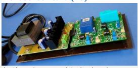
Single Phase Sensor card is developed to sense 01 AC/DC Voltage, 01 AC/DC Current Signals. It is possible to add offset voltage for interfacing sensed signal with unipolar ADC, amplitude calibration is also possible. More than Two Single Phase Sensor cards can be cascaded with each other.
