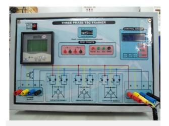
Trainer for studying three-phase Thyristor Switched Capacitor (TSC) operation. 3 banks of Thyristor switched capacitor with matching reactive load, AC switch (Thyristor-diode) for connecting and disconnecting capacitor banks.
