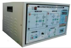
Trainer for studying half-bridge and full-bridge single-phase inverter circuits. Triggering scheme like square wave function, square wave sine PWM can be experimented.
