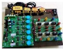
Three Phase Thyristor Firing Card basically consists of three Zero Crossing Detection Circuit and six pulse transformer based Thyristor gate circuit drive. Three Phase Thyristor Firing Card have two control as Analog control and Digital control.
