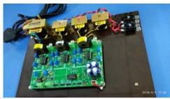
It senses 03 AC Voltage, 03 AC Current Signals. Also, 01 DC Current and 01 DC Voltage measurement is possible. It is possible to add offset voltage for interfacing sensed signal with unipolar ADC, Amplitude calibration is also possible. Quadrature Encoder Interface section is provided. Hall Sensor or Encoder Interfacing for Three channels to connect either three lines of hall sensor or A-B-Z pulses of encoder is provided.
