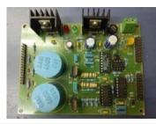
Thyristor Firing Card basically consists of Zero Crossing Detection Circuit and pulse transformer-based Thyristor gate circuit drive. Output of ZCD circuit is given to Microcontroller as input (on Interrupt pin).
