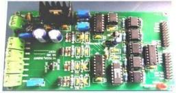
SPI Based ADC-DAC module is equipped with 13-bit SAR ADC and 12-bit DAC ICs, developed for fast data acquisition applications. The MCP3302 is 13-Bit 4 single ended/2 Differential channel Low Power A/D Converter with High Speed SPI Serial Interface. The module has MCP 4822 12-Bit DAC with Internal Voltage reference and High Speed Serial Peripheral Interface. Data are transferred serially via the 3-wire bidirectional SPI bus.
