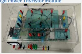
Three Phase Thyristor Power and Driver Card with Sensing circuit and 1200 V, 30 A Thyristor Modules.
