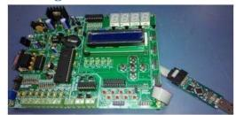
NI ATMEGA32 is a development kit with AVR microcontroller. AVR controller has up to 32KB flash size and 2KB of internal RAM. All I/O ports of the controller are available on the expansion bus thereby increasing the options for interfacing other devices.
