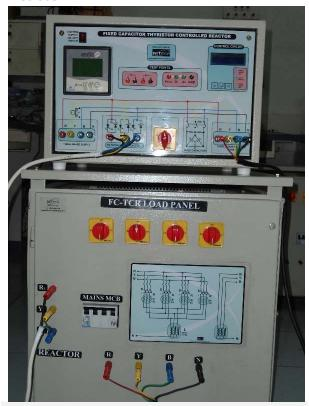
Trainer for studying three-phase Thyristor Controlled Reactor working with fixed capacitor (FC-TCR). Reactive load bank with fixed capacitor and Thyristor Controlled Reactor is provided.
