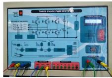
This trainer is for studying Three Phase PWM Rectifier Operation. Experiment setup consists of three-phase PWM rectifier, 32-bit Cortex M4 ARM microcontroller based controller for gate pulse generation, and load. Test points for current and voltage waveform observation across different elements are provided.
