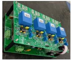
Four channel sensor card for measuring four AC/DC voltages. Hall effect voltage sensors are used. Outputs are scaled to 0-3.3V to directly connect ADC of microcontroller. Auxiliary power supply and required connectors for power connections are provided.
