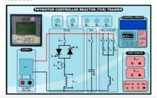
Trainer for studying working principle of single phase Fixed Capacitor Thyristor Controlled Reactor (FC-TCR). It provides inbuilt reactive load arrangement and fixed capacitor firing circuit, loading and power circuit with proper isolation.
