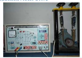
Trainer for studying Sinusoidal Pulse Width Modulated (SPWM) as well as Space Vector Modulated (SVM) inverter fed variable frequency drive operation.
