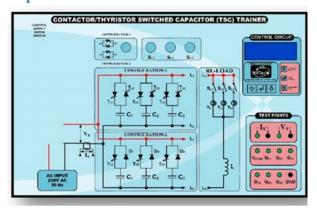
Trainer for studying working principle of single phase Thyristor Switched Capacitor (TSC). Trainer provides load panel with reactive load arrangement and fixed capacitor banks.
