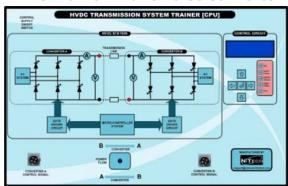
Trainer to demonstrate principle of operation of HVDC transmission system. The experiment setup consists of converter station and inverter stations, made using six-pulse converters for making bipolar configuration of HVDC. Bidirectional control of power can be experimented
