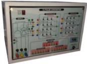
Trainer for studying principle operation of 12pulse converter. Star-Delta step-down transformer, Uncontrolled and controlled rectifier power configuration is provided. Provision for gate pulse observations and isolated current waveform observation is provided.
