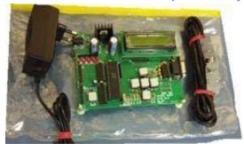
8051 Microcontroller @ 18.432 MHz, Flash Memory, Buffered port pins with indication LEDs, 6 clock mode, and 16x2 LCD Display, 5 keys, RS-232 communication support for ISP. Necessary IDE and ISP utility.
