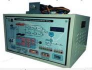
Trainer designed for studying sensored and sensorless control of Permanent Magnet Synchronous Motor (PMSM) drive operation.
