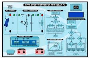
Trainer for studying MPPT boost converter for solar PV module. Boost converter operation in open-loop/closed-loop. Plotting PV characteristics, MPPT methods can be experimented.
