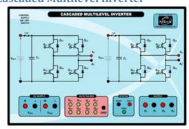
Trainer for studying 5-level cascaded multilevel inverter formed by cascading two H-bridges. The kit includes following three components:
