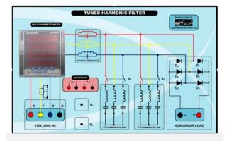
Trainer for studying tuned harmonic shunt passive power filter operation. Non-linear load along with bank of 5<sup>th</sup> and 7<sup>th</sup> harmonic is provided.
