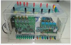
High-power four-leg inverter module with independent IGBT, driver circuit, sensor circuit and protection circuit.
