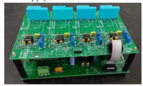
Four channel sensor card for measuring four AC/DC currents. Hall effect current sensors are used. Outputs are scaled to 0-3.3 V to directly connect ADC of microcontroller. Auxiliary power supply and required connectors for power connections are provided.
