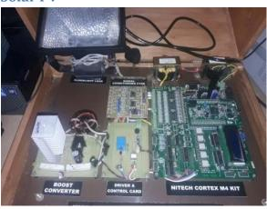
Trainer for studying MPPT boost converter for solar PV module. 450 W Boost Converter for MPPT.
