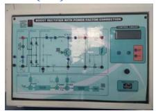
Trainer for studying operation of Boost Rectifier with Power Factor Correction. Experiment setup consists of low voltage boost rectifier with PFC, 32bit Cortex M4 ARM microcontroller based controller for gate pulse generation, and load. Test points for current and voltage waveform observation across different elements are provided.
