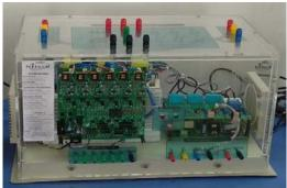
High Power IGBT Inverter Module is developed with Protection and Sensing circuit. High Power Inverter Module is intended to quickly implement a digitally controlled; six switch DC/AC inverter, supporting both solar and renewable energy types of applications as well as standalone Sine Inverter designs. It can also be used for power quality improvement solution like reactive power compensations using different topologies.
