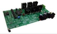
Three Phase H-Bridge Card is a ready to use hardware with six IGBTs connected in bridge configuration. Six gate pulses generated with microcontroller can be interfaced with this card. This Card can be used for designing applications like ac induction motor drive, BLDC drive or as a standalone three phase inverter. This module is designed with optical isolation between the controller card and the inverter bridge to be used for projects in power-electronics.
