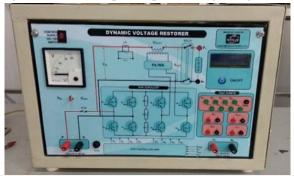
Trainer for studying static voltage regulation using dynamic voltage regulator (DVR). configuration of single phase voltage source inverter to inject voltage in series. Isolated observation of injected voltage, load voltage and load current waveform impossible.
