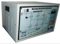
Trainer for studying 120 degree, 180 degree, Sine PWM, SVM controlled three-phase inverters. The kit provides platform for various experimentation on three-phase inverters.
